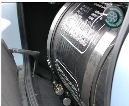
The HyCar is operated with gaseous hydrogen. This hydrogen is stored in two high-pressure tanks at a pressure of 200 bar. Each tank features a gastight interior tank made of aluminium which is wound with carbon fibres and weighs 32 kg. This means that 76 litres of hydrogen can be stored per tank. The vehicle is refuelled using the HyStation for instance, and the refuelling operation is thus as safe and convenient as on a conventional vehicle.
