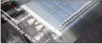
The fuel cell system is accommodated beneath the glass load floor in the HyCar's tail. This allows a view of this novel drive technology.
