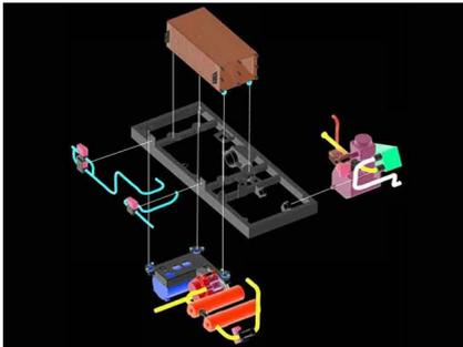
The fuel cell system was the actual focus of the project. ESORO developed the entire system around a bought-in fuel cell stack. This included the entire conception, evaluation of the various components and dimensioning them, system integration in the vehicle, development of the monitoring and control system for fully automatic operation and, finally, implementation and testing of the system.
